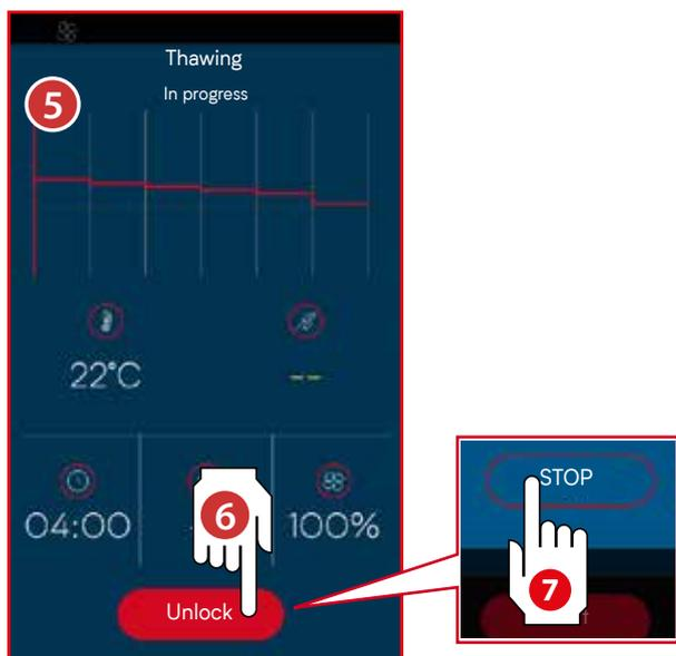
**5** After tapping the word **Start**, defrosting begins and will end when the set time has elapsed.
